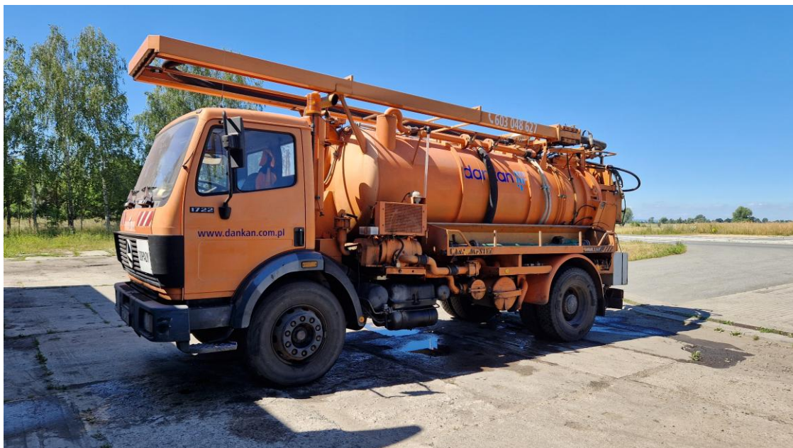
Septic tanker truck Source: Dankan Sp. z o.o.
